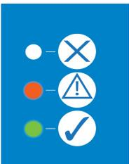
When the filter is full/blocked, the red LED on the control panel will illuminate. All three LEDs will be illuminating as shown below. A filter change is required at this stage.
