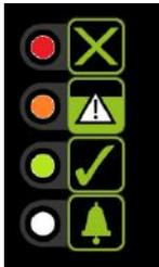
If the VOC (Volatile Organic Compound) alarm option is installed in your PrintPRO 800 DS, the extractor will monitor and detect the level of VOC particles in the air. If the VOC level rises above a pre-set level then the LED to the right of the bell symbol will flash red. This requires the replacement of the Combined filter.
