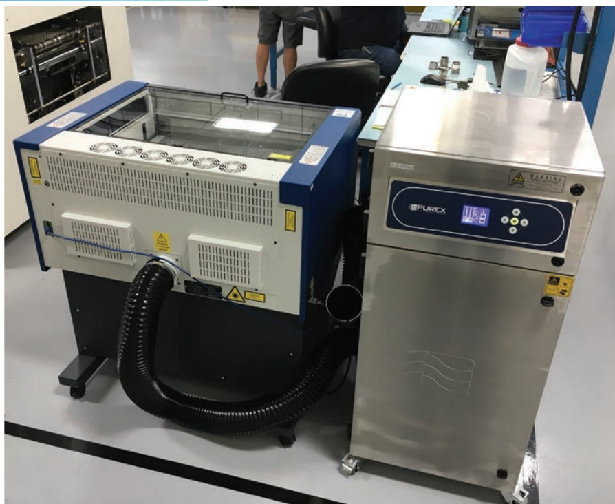
In regard to power consumption, extractors typically require the same power as the host machine. (Image courtesy Purex Fume Extraction by BSE)
